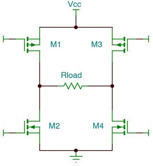
Figure 10. Simplified BTL Output Stage
