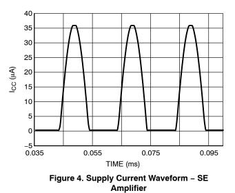
Current is only delivered for a half cycle in an SE configuration due to the nature of the half bridge output.
