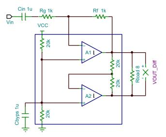
Figure 6. Bridge Tied Load (BTL) Amplifier
