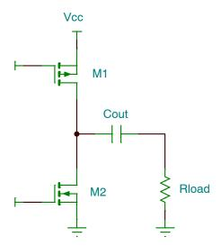
Figure 5. Class B Output Stage – SE Amplifier
